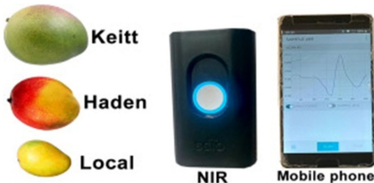
Figure 1. General setup for scanning and the three mango varieties.
