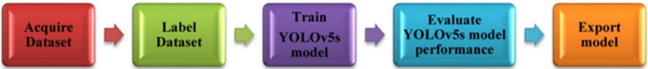
Figure 2. Procedure for developing and implementing a YOLOv5s-based crop and weed classification scheme.
