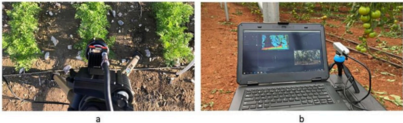
Figure 1. A sample of the gear utilized for ground-based field data capture: (a) an RGB imager equipped with a C-mount lens; and (b) a laptop linked to an RGB depth camera.
