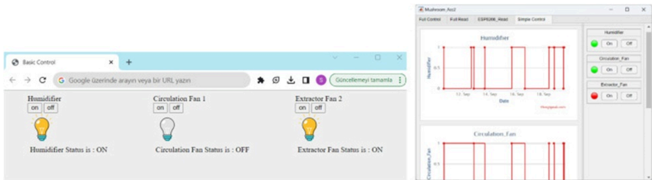
Figure 10. Basic control node user interfaces (a) Web page (b) MATLAB application.
