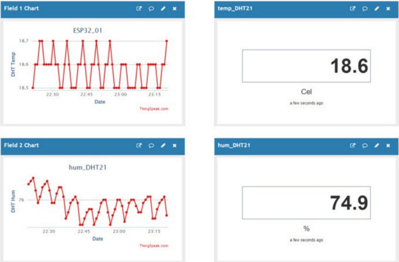
Figure 18. ThingSpeak IoT platform interface of DHT21 sensor (25 Mar 2023).
