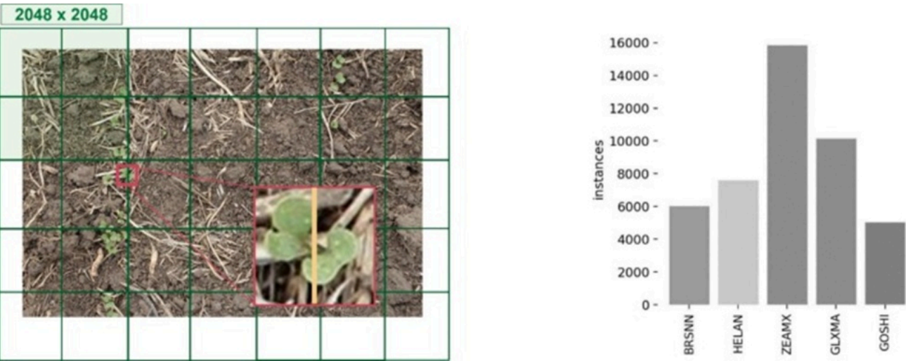
Figure 9. Left) The image is tiled into 2048 × 2048 patches, as shown. An overlapping stride window of 1024 × 1024 is applied after padding the image to get a fixed tile size for every stride. Right, the total number of instances of objects used as input to the training step is shown by class.
