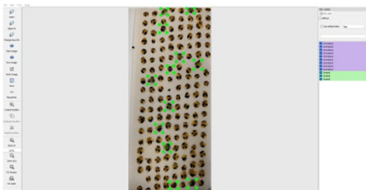
Figure 3. Data labeling using the LabelImg graphical user interface. Tight bounding boxes for the two classes were drawn over the damages present to set the ground truth.
