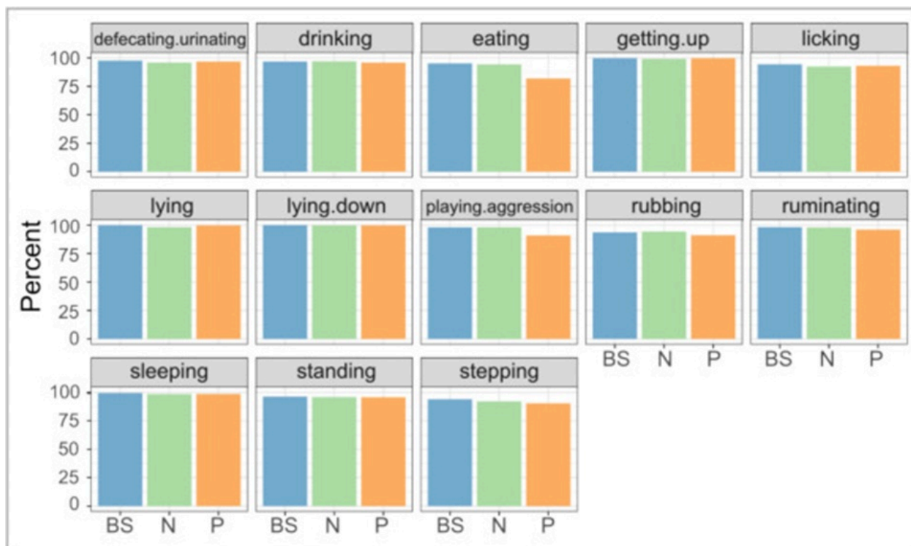
Figure 14. F1 Score values of the RandomForest classifier with different sensors: both sensors (BS), Noseband (N), and Pedometer (P) with settings Padding = 3; Window = 10 and Train size = Validation size = 0.5. Most movements were better recognized with the noseband than with the pedometer.
