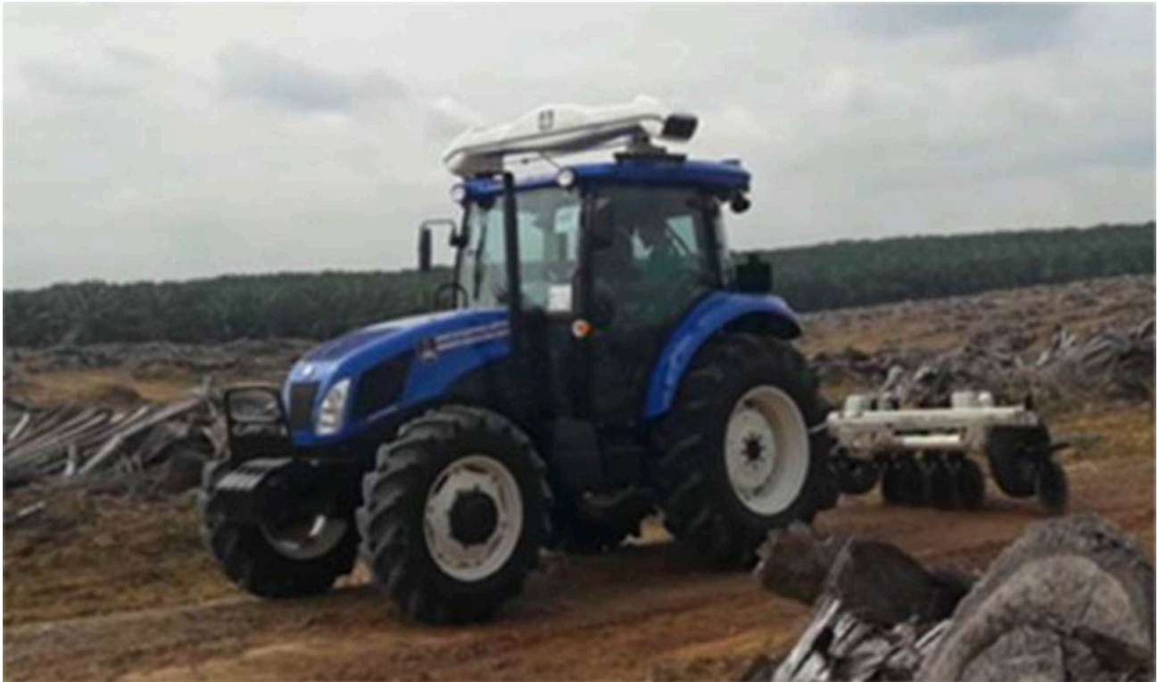
Figure 2. A tractor with an autopilot system is traversing the experimental field.
