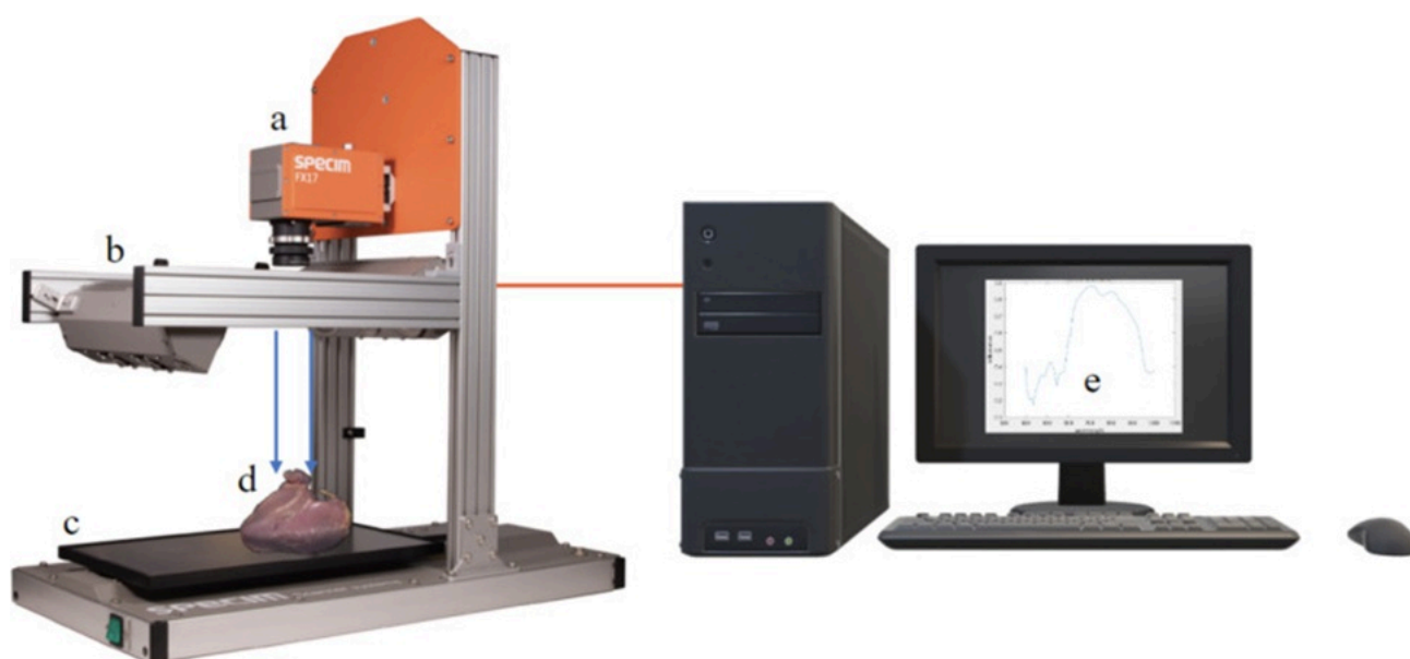
Figure 3. Hyperspectral imaging system setups: a) SPECIM FX 10e camera, b) Halogen illumination, c) Conveyor, d) chicken breast Sample, and e) spectral reflectance graph.
