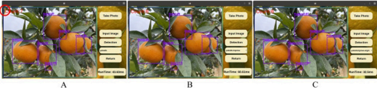
Figure 21. Comparison of detection results under edge device deployment: A) Results with original YOLOv8n model deployment, B) Results with improved YOLOv8n model without TensorRT-optimized deployment, and C) Results with improved YOLOv8n model with TensorRT-optimized deployment.
