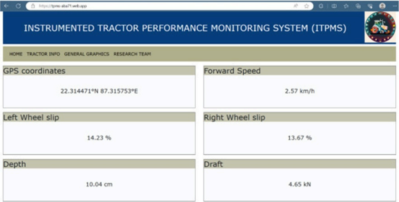
Figure 5. Real-time data monitoring of the instrumented tractor’s performance parameters on the web interface.
