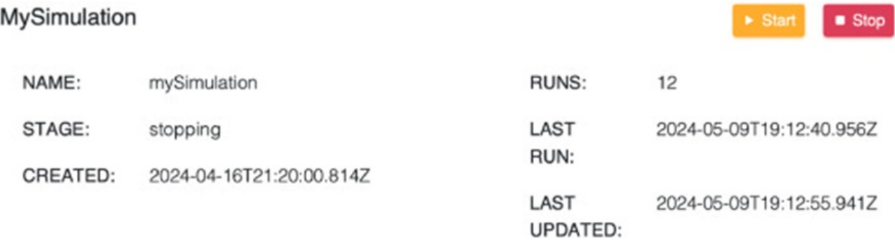
Figure 7. Emulation of a live IoT sensor tasked with stochastically generating values mapped to the HR attribute.
