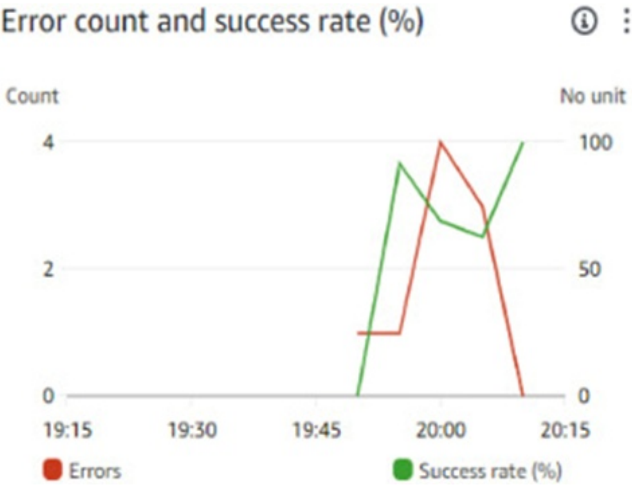
Figure 12. Lambda operational output portraying fault ratios and success ratios under data ingestion load for scenario 2.
