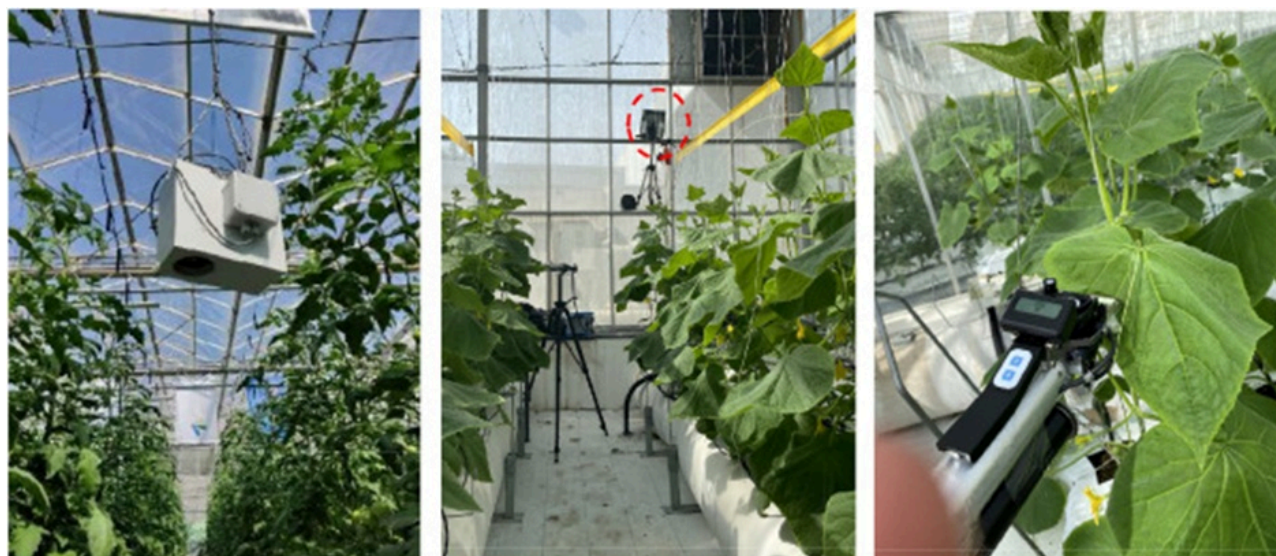
Figure 1. Equipment used for data collection in the greenhouse: a) Aspirator box, b) Hyperspectral camera, and c) Gas exchange measurement system.
